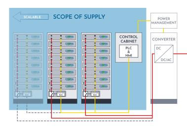
High-quality and inherent safe LFP battery cells and a permanent monitoring by Battery Management System on cell, module and on rack level guarantees the highest standards for safety. LFP battery chemistry does not catch fire during thermal runaway, short-circuit or mechanical damage which makes the COBRA system the safest solution for the use at sea where safety is essential.
